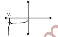
c) Because of heavy doping width of the depletion layer decreases, the electric intensity in the depletion layer increases Zener breakdown is pulling the electrons from valence bonds by the action of this strong electric field.
